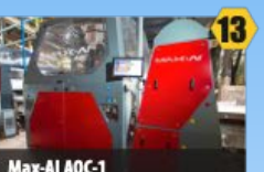
Max-AI AQC-1 AI-powered robotic sorter recovers recyclables from residue line
