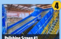
Polishing Screen #1 Separates 6-12" material into different fractions: mixed paper, containers, fines
