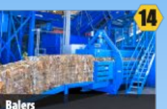
Balers Compresses recyclables into bales
