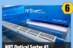
NRT Optical Sorter #1 Uses high-res color detection to recover small cardboard
