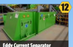
Eddy Current Separator Captures aluminum
